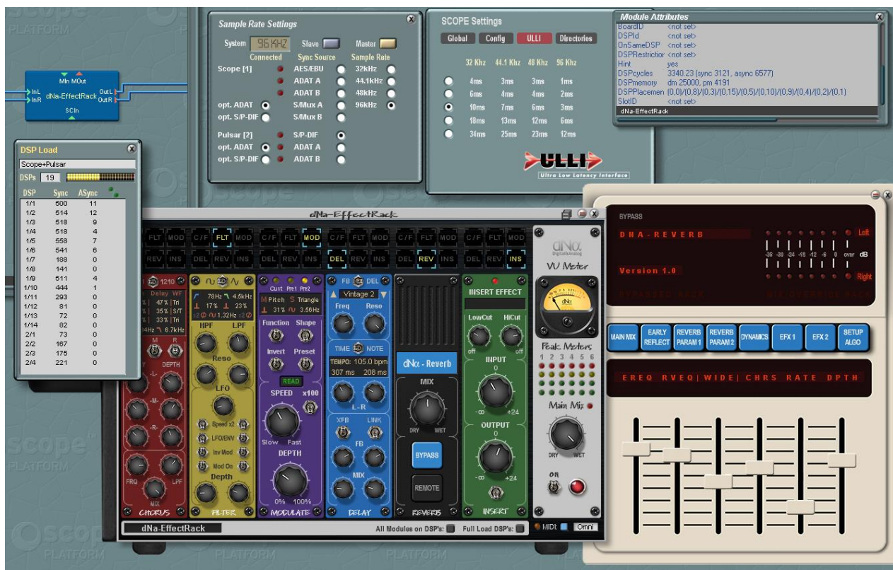
dNa-EffectRack running at 96kHz with moderate ULLI on a Pulsar1 + Scope SRB PCI Card.
