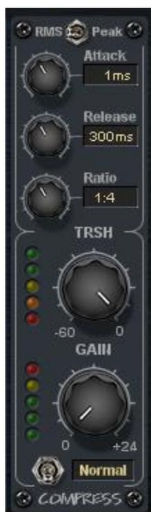
**RMS/Peak:** Controls how the compressor behaves, more like a compressor in RMS mode or faster for limit purposes in the Peak mode. Let your ears and your logic decide.
