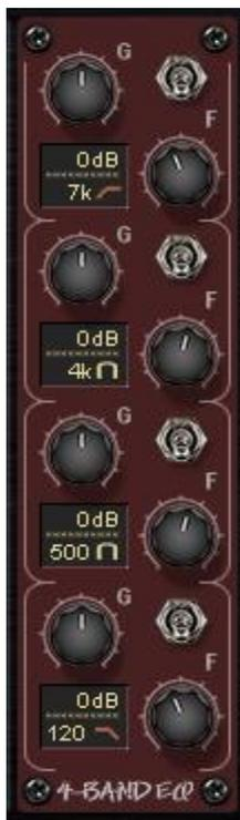
**“G” Rotary knobs:** Controls the GAIN of each band in 2dB steps, going from a minimal of -18dB to a maximum of +18dB, values also show in the small display.
