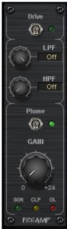
**Drive:** Uses a drive/softclipping circuit to add warmth and coloration to the signal.
